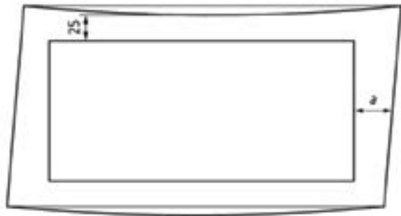
Figure 1 : Measuring of flatness
